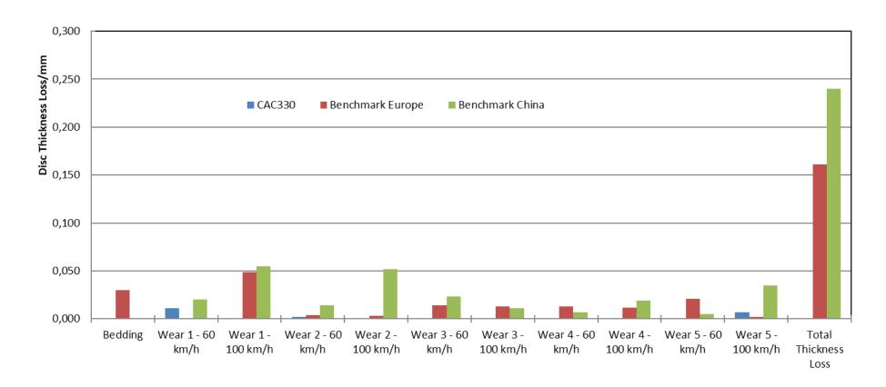
Kyoto Japan's disc wear performance is the best among the three samples, the brake disc is barely damaged after ISO 26866 test.
