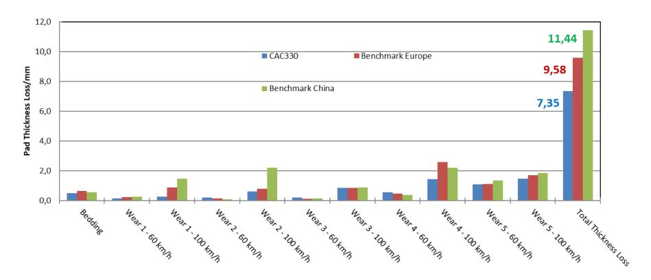
Kyoto Japan CAC330 has the best wear performance among the three samples with an ISO 26866 experimental wear of only 7.35mm.
